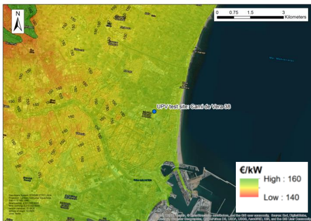
Figure 7 - Estimated savings between double-U system and Cheap-GSHPs coaxial one expressed as €/kW for Valencia
