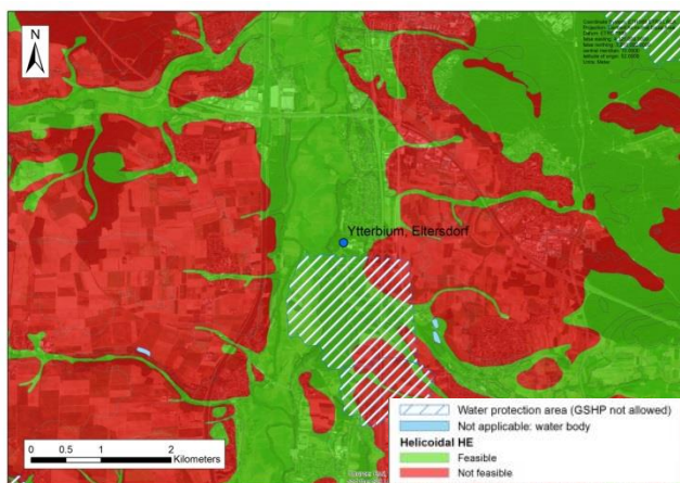
Figure 5 - Helicoidal HE feasibility map for Erlangen
